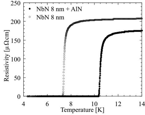
**Figure 4.** R-T curves of the NbN films on the quartz wafer with and without the AlN buffer layer.
