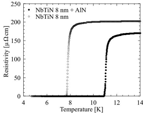
**Figure 2.** R-T curves of the NbTiN films on the quartz wafer with and without the AlN buffer layer.
