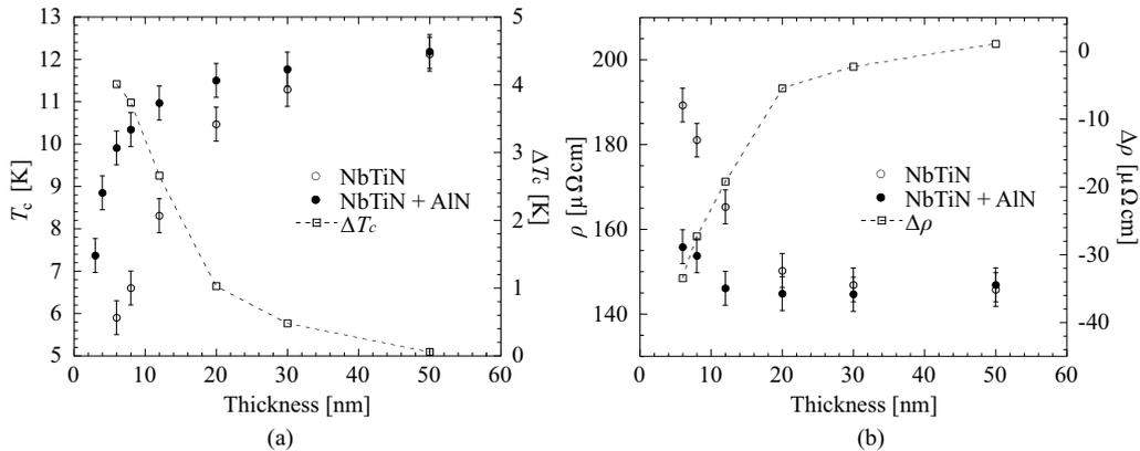
**Figure 3.** Thickness dependence of  $T_c$  (a) and resistivity (b) for the NbTiN film on the glass wafer with and without the AlN buffer layer. Dashed lines represent the difference.
