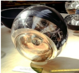
Optical Module (10" PMT in 17" glass sphere) photon detection
