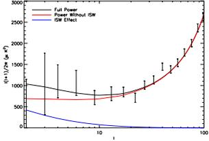
Figure 1. Power spectra of temperature anisotropies. We show the full power (black), power without ISW effect (red) and power for late ISW (Blue) only. The error bars come from WMAP 7-year results. The ISW effect manifests itself on large angular scales because the CMB temperature fluctuations are dominantly induced by gravitational potential at large scales.
