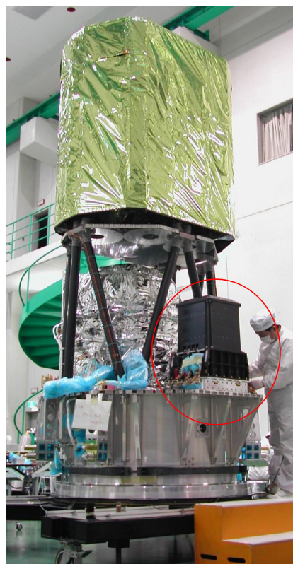
図 7.1 b: The Suzaku spacecraft under construction, carrying the Hard X-ray Detector sensor part (red circled).
