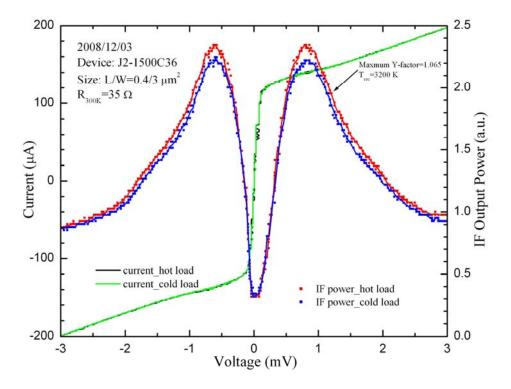
Figure 1 I-V curve and IF response of the waveguide 1.5 THz HEB mixer (Jiang et al.)
