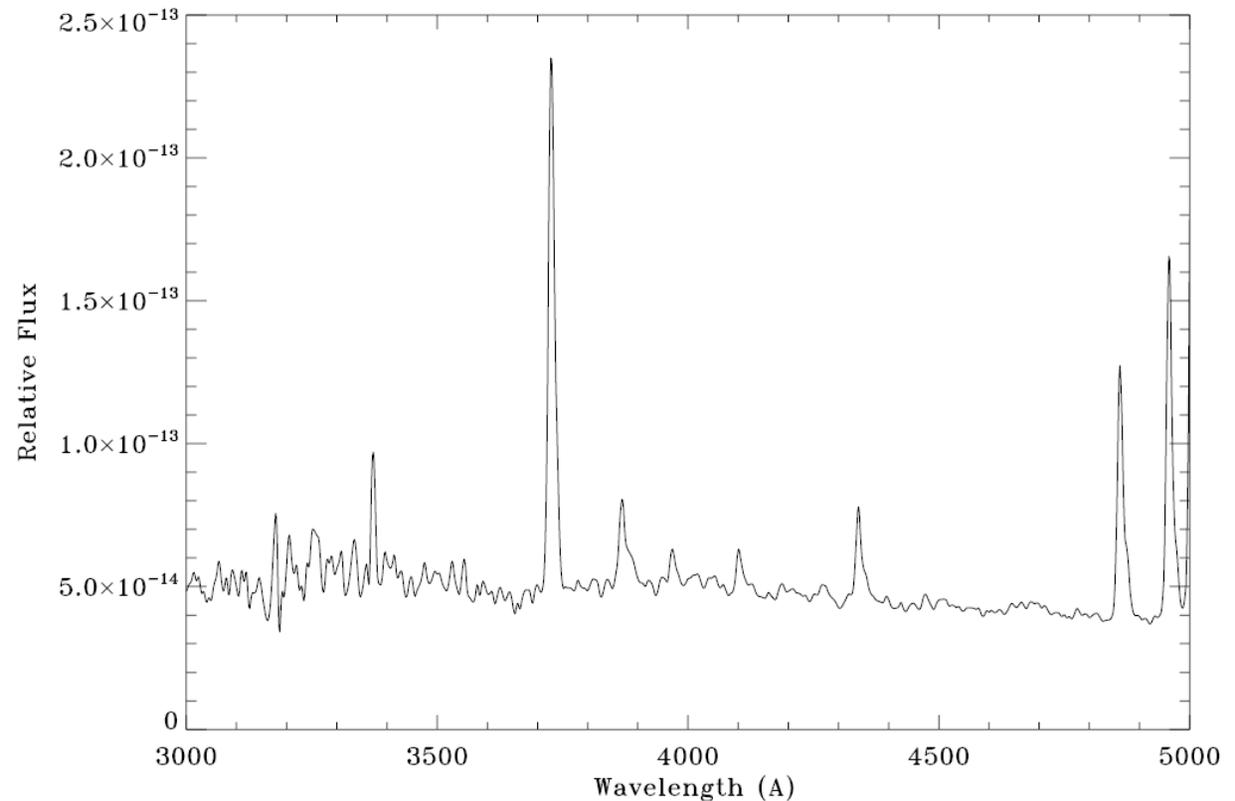
Flux in each spectral bin in spectrometer will depend on width of the spectral bin and which part of the galaxy spectrum it is sampling.
