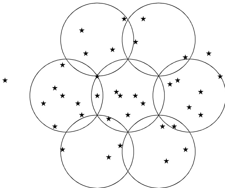
Patrol Region – Area of the focal plane accessible to one fiber (9.5 mm diameter)
