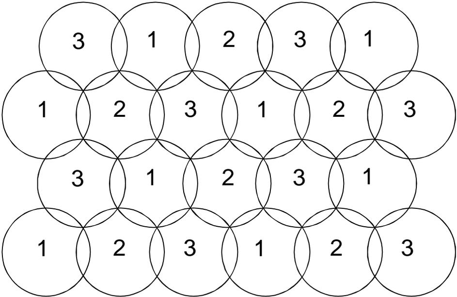
The science fibers are back-lit in a sequence to allow discrimination between fibers in the overlap regions between adjacent fibers.
