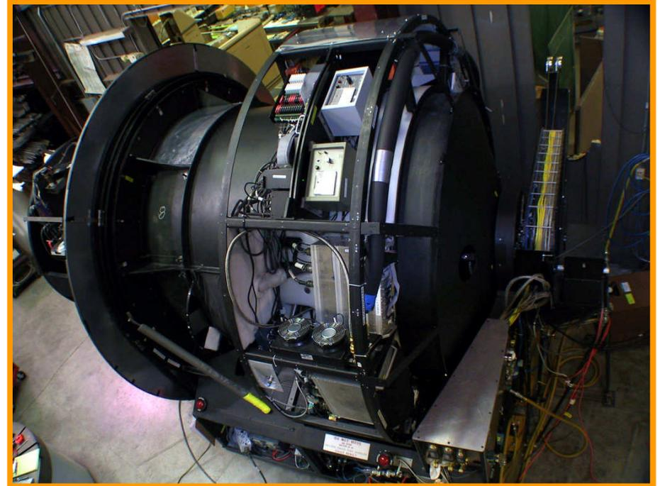
DEEP2 : Typically 120 simultaneous spectra over  $16.7 \times 5'$  field using mechanically fabricated slit masks
