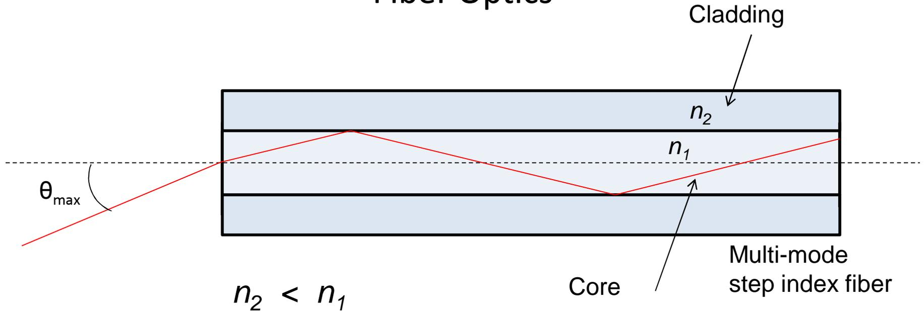
There is a maximum angle,  $\theta_{max}$ , called the acceptance angle, for which light entering the fiber will propagate through total internal reflection. This angle is defined by:
