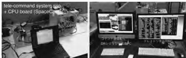
図 7.14: Digital electronics and command/telemetry software of the HXI/SGD on test.
