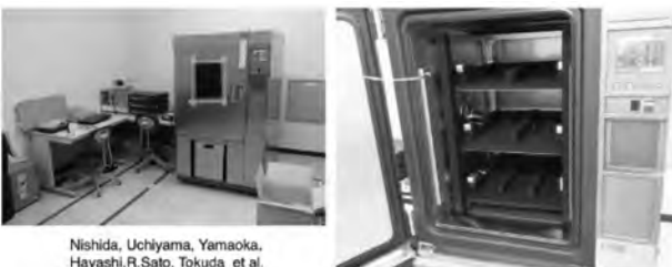
図 7.11: Set-up at MHI Komaki factory for measuring the flight model BGO units.
