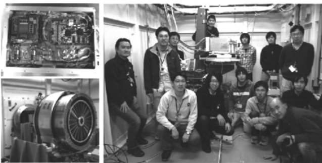
図 7.13: Tests at SPring-8 (right), where a Hard X-ray Telescope (left bottom) was combined with DSSD for the HXI (left top).
