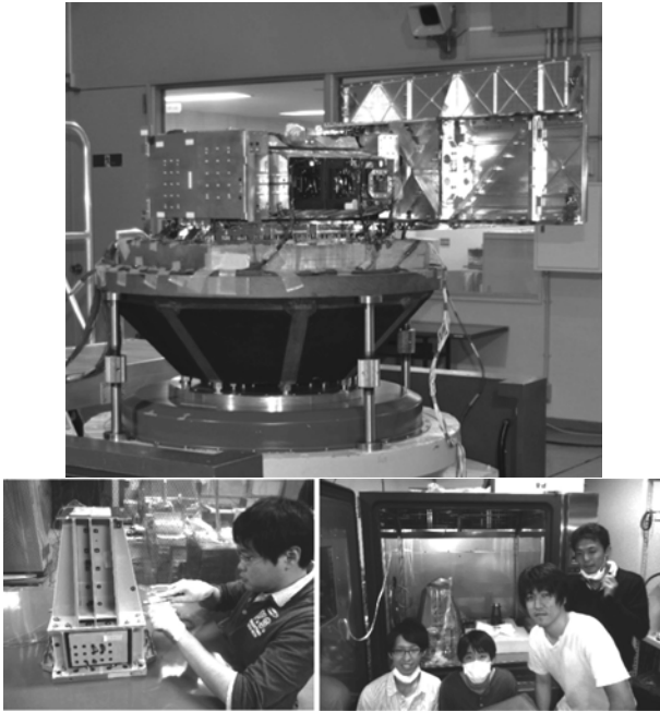
図 7.10: (Top) SGD-S EM housing vibration tests at Tukuba/JAXA. (Bottom) HXI-S EM thermal distortion test at ISAS/JAXA.
